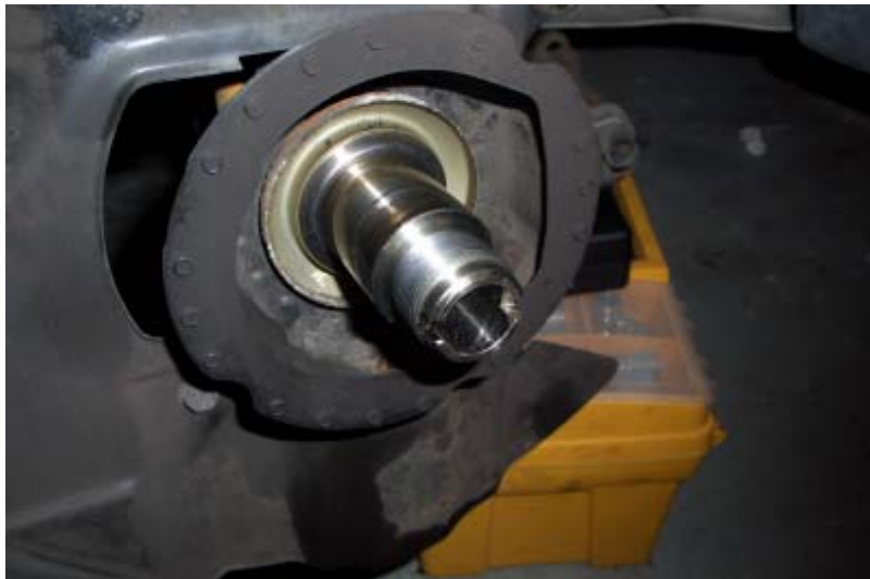
Exposed Axle Stub
